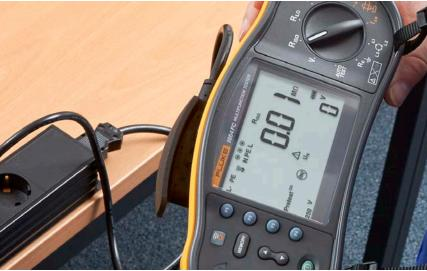
If the tester detects that an appliance is connected, it will stop the insulation test and provide a visual warning. This helps eliminate accidental damage to peripheral equipment and keeps your customers happy.
