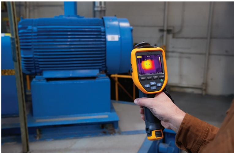
Infrared thermography offers the possibility to detect small or developing problems before they lead to failures. In industrial applications, some problems show up through unusual vibrations or noises, but other problems do not show these symptoms. Many electrical problems can be identified by their thermal patterns, which, if not detected, can lead to equipment failure or an even more serious electrical hazard.
