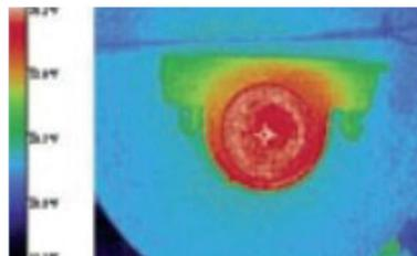
**4. Checking electric motors** (Fig. 4)
