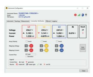
Setup + connection + controls via PC/Mac (no on-board screen)
